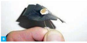
Then test whether the switching works for each device by covering and uncovering the photoresistors with your hand.
